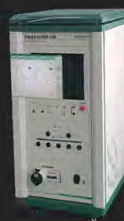
• 10kV 5kA Surge Test
