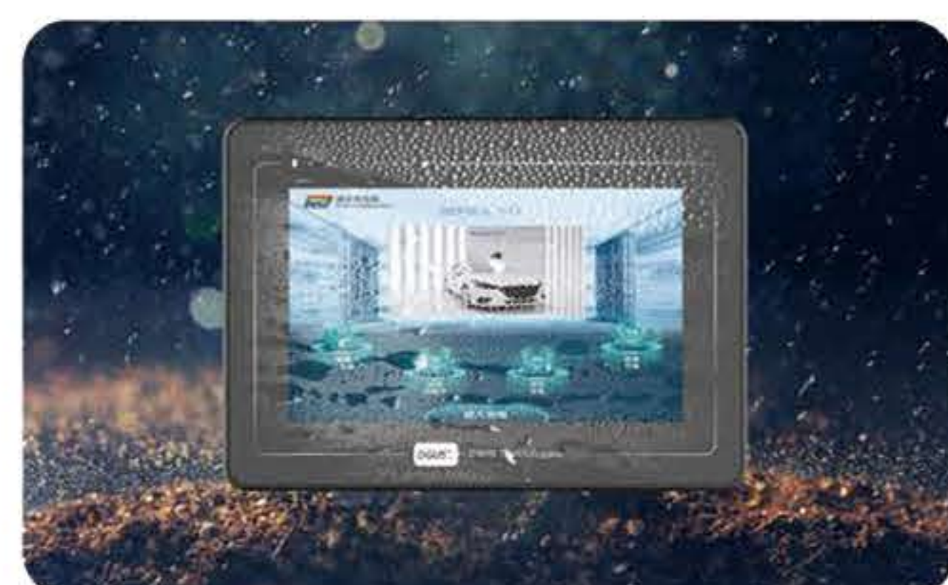
High Temperature & High Humidity Resistance (-40~85°C, 10%~95%RH)
