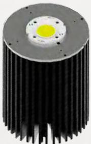
Citizen CITILED High Bay LED cooler with CoolTube® heat tube and direct mounting holes for Mean Well HBG series driver
