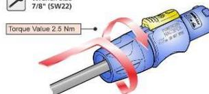
E Fasten bushing by means of a fork wrench 7/8" (SW 22), min. Torque 2.5 Nm (1.8 lb-ft).
