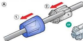
A Place the bushing (1) and the chuck (2) over the cable.
