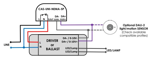
Note: The internal relay is normally closed (NC). When the controller is unpowered, LOUT is connected to L.
