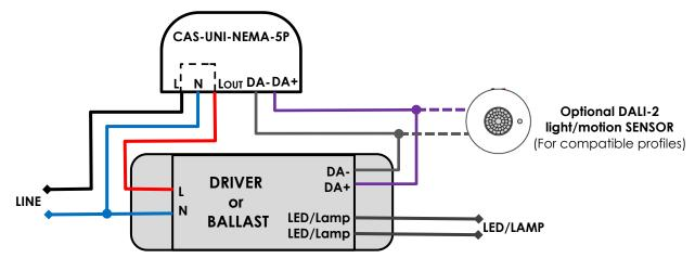
Note: LOUT is permanentlyconnected to L through an internal link
