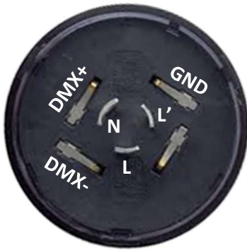
BOTTOM VIEW Note: L input and L' output are internally shorted together inside CAS-UNI-NEMA-DMX
