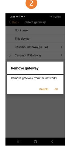
A pop-up will appear to enable the removal of the gateway. Tap on Ok to remove it or on Cancel to cancel the removal.
