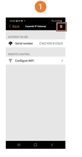
Tap on the trash can icon to remove the gateway from the network.
