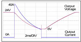
Peak load 40A (resistive load) for 5ms Output voltage dips from 24V to 6V.
