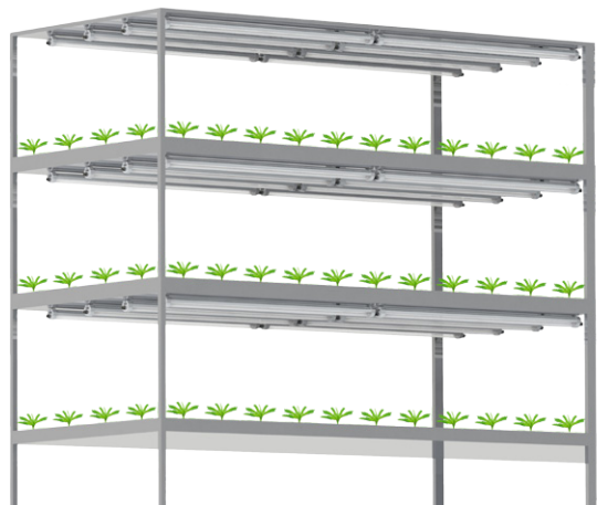
Grow rack setup vegetative growth 8 lamps per canopy layer in 4 daisy-chain lines with reduced cabling PPFD 420 \mu mol/sm 2
