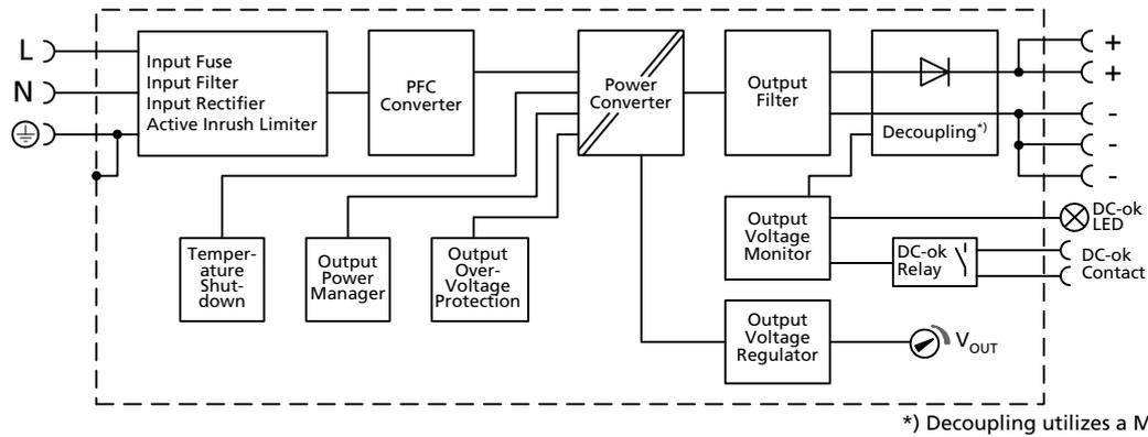
Fig. 12-2 Functional diagram CP10.241-R2
