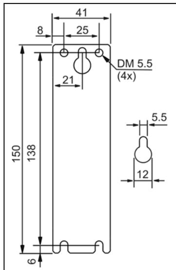
Fig. 24-6 **Wall/panel mounting, side view**
