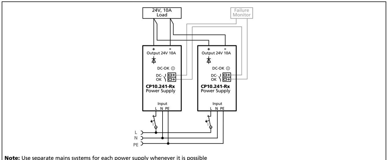
Fig. 25-8 **Wiring diagram, N+1 Redundancy for 20A output current**
