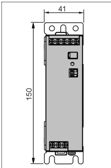
Fig. 24-5 **Hole pattern for wall mounting**
