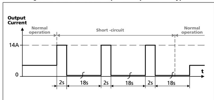
Fig. 6-3 **Dynamic overcurrent capability, typ.**
