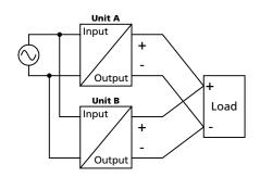
Energize all units at the same time. It also might be necessary to cycle the input power (turn-off for at least five seconds), if the output was in overload or short circuits and the required output current is higher than the current of one unit.
