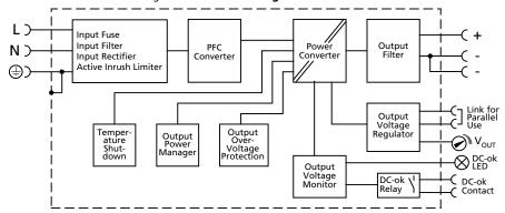
Fig. 11-3 Functional diagram CP20.241-V1
