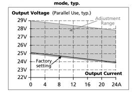
Fig. 6-2 Output voltage in "parallel use"
