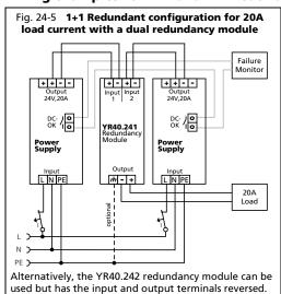
supplies and redundancy modules Monitor +-+-+ + - -Output +-+-++--Output Input Inpu 24V.20A 쭚 DCok 시 YR40.241 YR40.241 Reaum Module Power Supply Power Supply */*// - | + L N PE /<del>//</del> - + L N PE 60A Load Alternatively, the YR40.242 redundancy module can be used but has the input and output terminals reversed.
