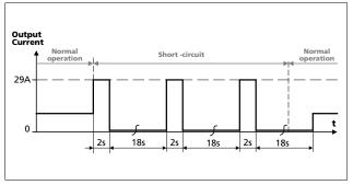
Fig. 6-4 Dynamic overcurrent capability, typ.
