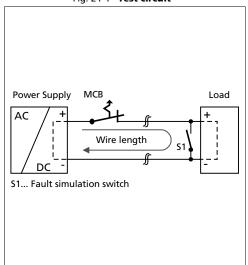
Maximal wire length\*) for a fast (magnetic) tripping:
