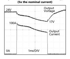
Fig. 24-2 100A peak current for 5ms, typ.
