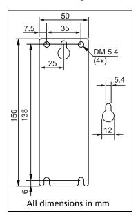
Fig. 23-6 Wall/panel mounting, side view
