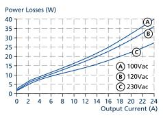
Fig. 9-2: Losses vs. output current at 24V, typ.
