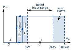
Fig. 3-1: Input voltage range
