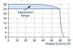
Fig. 6-2: Dynamic overcurrent capability, typ.
