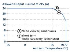
Fig. 16-1: Output current vs. ambient temp.  $(I_{nom} = 20A; I_{out} \text{ with PowerBoost} = 24A)$
