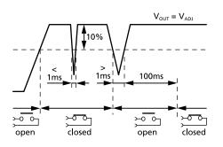
Fig. 8-1: DC-ok relay contact behavior
