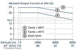
Fig. 16-2: Output current vs. altitude
