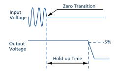
Fig. 7-2: Shut-down behaviour, definitions
