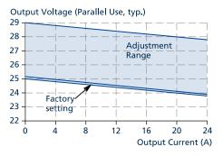
Fig. 6-4: Output voltage in "parallel use" mode, typ.
