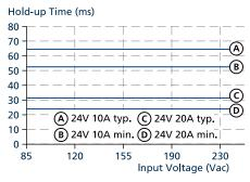
Fig. 7-1: Hold-up time vs. input voltage
