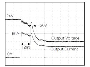
Fig. 24-3: 60A peak current for 12ms , typ. (3x the nominal current)
