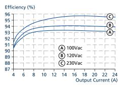
Fig. 9-1: Efficiency vs. output current at 24V, typ.
