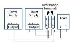
Fig. 13-1: Using distribution terminals
