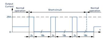
Fig. 6-3: Short-circuit on output, Hiccup<sup>PLUS</sup> mode, typ.
