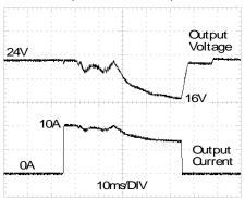
Fig. 23-3 15A<sub>peak</sub> current for 12ms, typ. (3x the nominal current)
