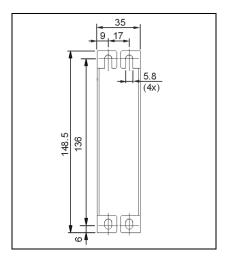
Fig. 22-6 Wall/panel mounting, side view
