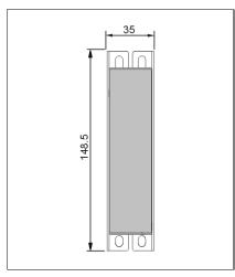
Fig. 22-5 Hole pattern for wall mounting
