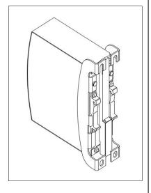
Fig. 22-4 Wall/panel mounting, front view
