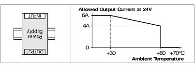
Fig. 23-9 Mounting Orientation C (Table-top mounting)
