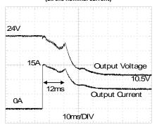
Fig. 23-2 **25A**<sub>peak</sub> current for 5ms , typ. (5x the nominal current)
