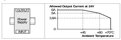
Fig. 23-8 Mounting Orientation B (Upside down)
