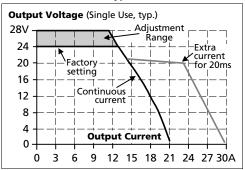
Fig. 6-2 Output voltage in "parallel use" mode, typ.
