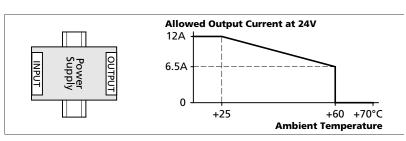
Fig. 22-14 Mounting Orientation E (Horizontal ccw)
