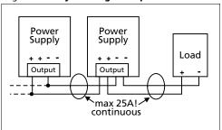
Fig. 11-2 Using distribution terminals
