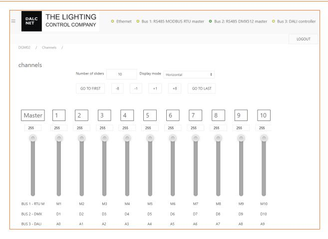
The DGM02 has a WebApp for the supervision and regulation of all the channels available in the various DALI, DMX, MODBUS protocols, which can be used from any device equipped with a compatible browser.
