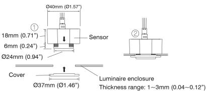
Assembly hole w/o cover: Ø25.4mm (1") Assembly hole with cover: Ø27mm (1.06")
