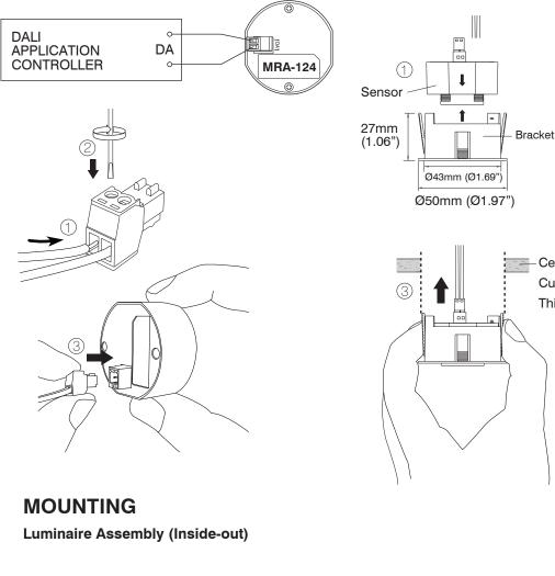
Ceiling Cut hole: Ø45mm (Ø1.75") Thickness range: 2~20mm (0.08~0.79")
