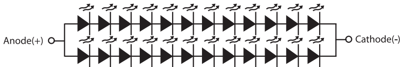
9W EdiPower® III HM Series Circuit Layout
