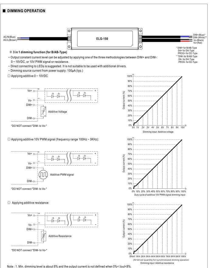
2. The output current could drop down to 0% when dimming input is about  $0k\Omega$  or 0Vdc, or 10V PWM signal with 0% duty cycle.
