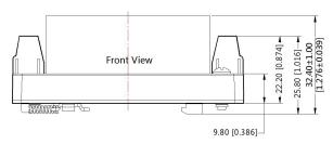
Note: Unit: mm[inch] Wire range: 24-12 AWG Tightening torque: Max 0.4 N·m Installed on DIN RAIL TS35 General tolerances: ±0.50[±0.020]
