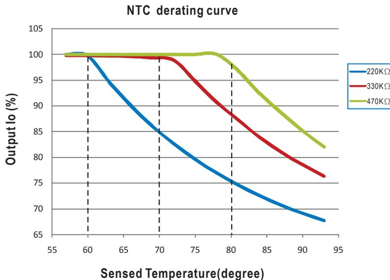
LCM-60EO have the built-in temperature compensation function ( $T \uparrow, I_o \downarrow$ ). By connecting a temperature sensor (NTC resistor) between the NTC +/- terminal of LCM-60EO and the detecting point on the lighting system or the surrounding environment, output current of LCM-40EO could be correspondingly changed to ensure the long life of LED.
