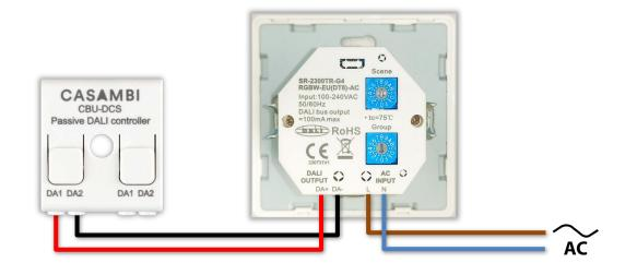
2. Use a flathead screwdriver to change the rotary selector of the "Group" and set it to "2".
