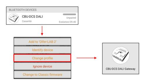
7. Add the CBU-DCS to the network where we want to control the devices with the touchpanel.
