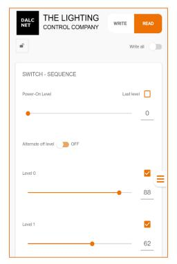
**Power-On level:** it is the intensity value to which the output is brought as soon as the device is powered if the switch is on ON. If the switch is OFF (open) the light will remain off.
