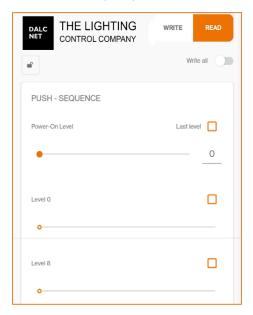
**Power On level:** it is the intensity value to which the output is brought as soon as the device is powered
