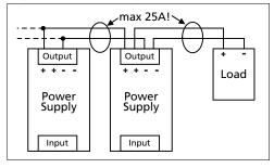
Fig. 22-4 Using distribution terminals
