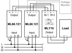
supply. In such a case, the defect unit becomes a load for the other power supplies and the output voltage can not be maintained any more. This can only be avoided by utilizing decoupling diodes which are included in the redundancy module MLY10.241.
