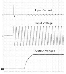
Input: 230Vac Output: 12V, 4.5A Ambient: 25°C
