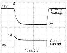
Peak load 9A (resistive load) for 50ms Output voltage dips from 12V to 7V.
