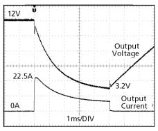
Peak load 22.5A (resistive load) for 5ms Output voltage dips from 12V to 3.2V.
