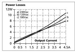
Fig. 8-4 Losses vs. input voltage at 12V, 4.5A, typ.
