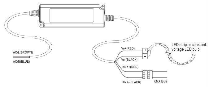
PWM KN series can be ETS adressing/programming WITHOUT connecting to AC mains
