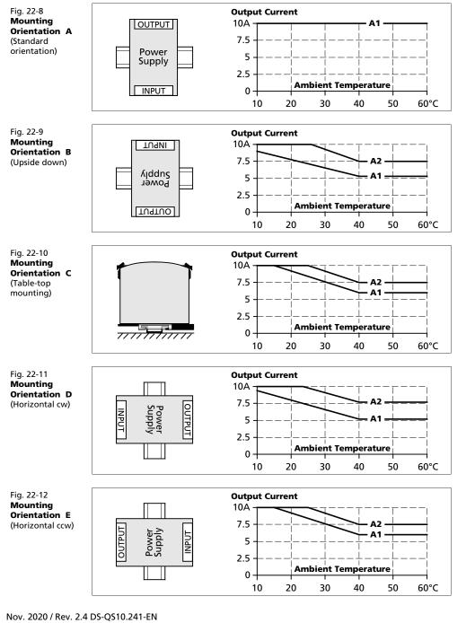
All parameters are specified at 24V, 10A, 230Vac, 25°C ambient and after a 5 minutes run-in time unless otherwise noted.
