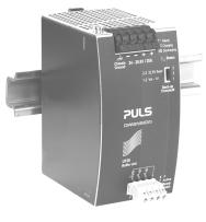
or extends the hold-up time after turn-off of the AC power. In times when the power supply provides sufficient voltages, the buffer unit stores energy in integrated electrolytic capacitors. In case of mains voltage fault, this energy is released again
