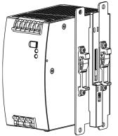
Side mounting with DIN-rail brackets
