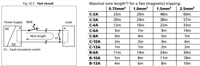
\*) Don't forget to consider twice the distance to the load (or cable length) when calculating the total wire length (+ and - wire).
