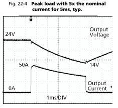
Peak load 20A (resistive) for 50ms Output voltage dips from 24V to 20.5V. Peak load 50A (resistive) for 5ms Output voltage dips from 24V to 14V.
