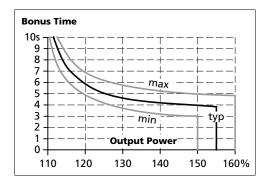
The BonusPower<sup>®</sup> is available as soon as power comes on and immediately after the end of an output short circuit or output overload.
