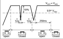
**Note:** The DC-ok feature requires that the output voltage reaches the nominal level after turn-on in order to function according to specification. If this level cannot be achieved, the overload lamp will be on and the DC-ok contact will be open. The overload signal will only shut off as soon as the adjusted voltage is reached.
