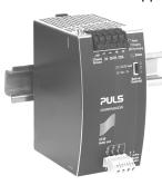
or extends the hold-up time after turn-off of the AC power. In times when the power supply provides sufficient voltages, the buffer unit stores energy in integrated electrolytic capacitors. In case of mains voltage fault, this energy is released again in a regulated process. One buffer module can deliver 20A additional current.
