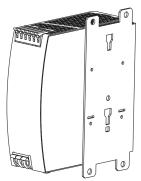
Side mounting without DIN-rail brackets
