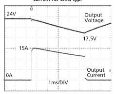
Peak load 15A (resistive) for 5ms Output voltage dips from 24V to 16V.
