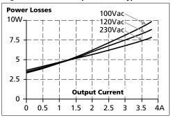
Fig. 9-4 Losses vs. input voltage at 3.8A, typ.
