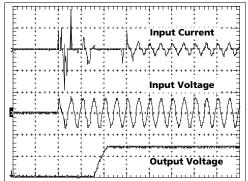
Input: 230Vac Output: 24V, 3.8A Ambient: 25°C
