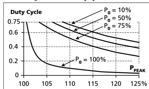
$$\text{DutyCycle} = \frac{T_{\text{peak}}}{T_{\text{peak}} + T_0}$$
