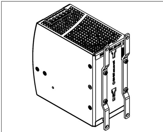
Fig. 20-2 Mounting Dimensions - Wall mounting bracket
