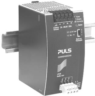
This buffer unit is a supplementary device for DC 24V power supplies and DC/DC converter. It delivers power to bridge typical mains failures or extends the hold-up time after turn-off of the AC or DC power. In times when the DC/DC converter provides sufficient voltages, the buffer unit stores energy in the integrated electrolytic capacitors. In case of mains voltage fault, this energy is released again in a regulated process.
