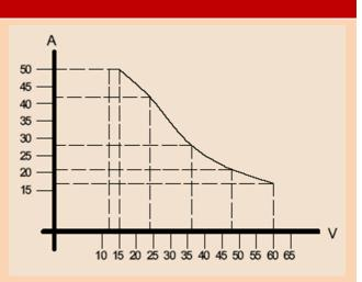
The RED00202A model can also be used smaller then 12Vdc. Please note that the DC-ok relay and the ADJ potentiometer will not function below 12Vdc.
