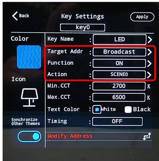
The rest of the buttons have to be configured in the same way in "Target Address" and "Function". In "Action" we will have to assign to each button the corresponding scene number, if the first button has been configured as "Scene0", the second button will be "Scene1", the third button will be "Scene2" and so on...
