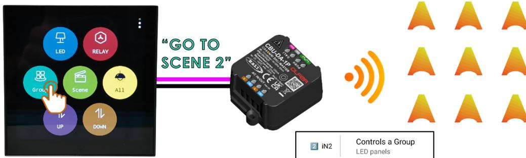
Then we could use the "UP" and "DOWN" buttons to dim that group of luminaires since it would be the last action activated.
