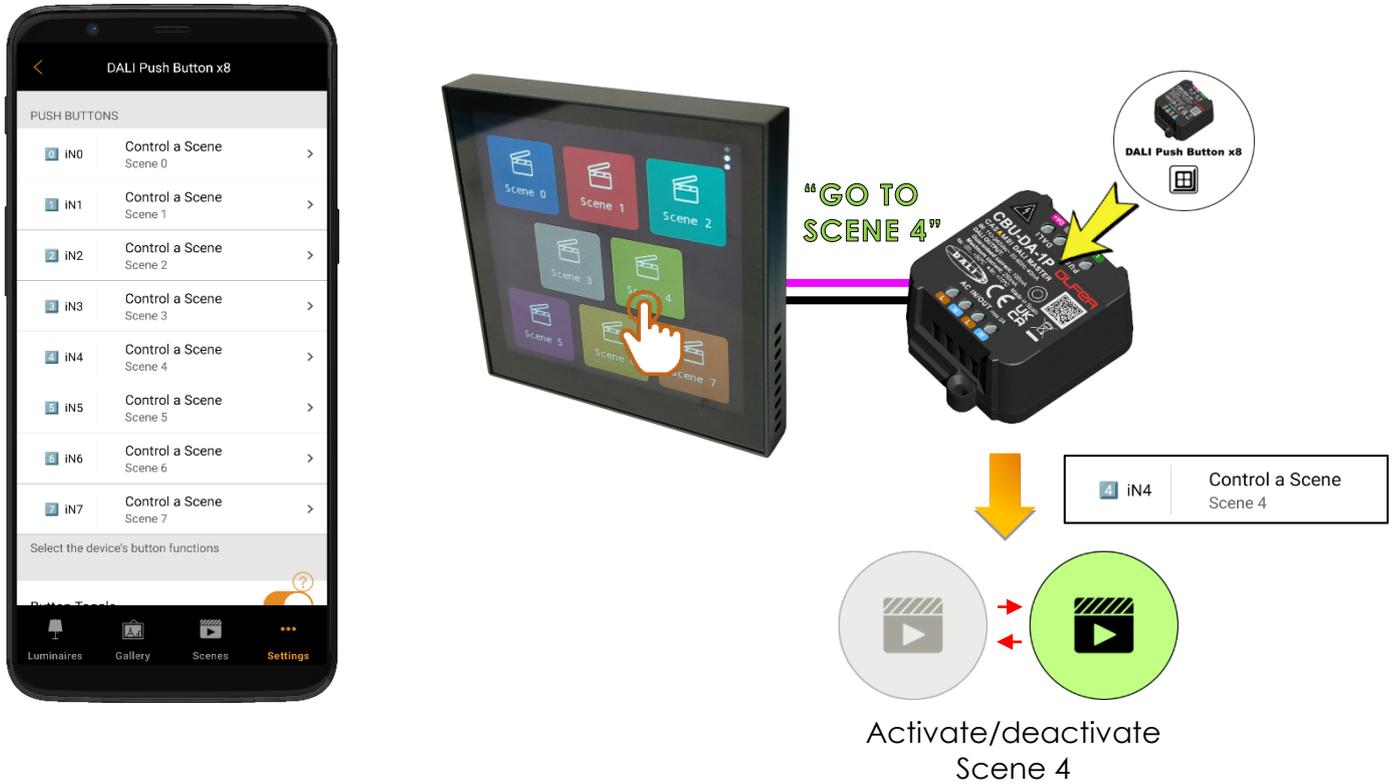
In this example all the buttons are configured practically in the same way: in "Target Address" they are set to "Broadcast" and in "Function" they are set to "ON". In "Action" we will have to assign the corresponding scene number to each button. In this case we have not included "UP" or "DOWN" buttons.
