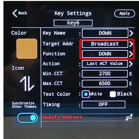
Again in "Target Address" we will set "Broadcast" and in "Function" we will configure one button as "UP" and another as "DOWN". In this case the parameter you have set in "Action" does not matter.
