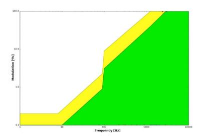
Thanks to the 4khz dimming frequency the SLIM-2CV-CASAMBI allows to reduce the Flicker phenomenon.
