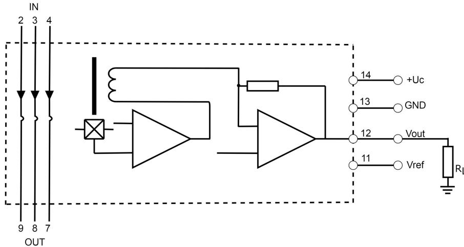
1.  $I_p$  is measured current. When the detected current is input from pin 2, 3 and 4, it is a forward current. When the detected current is input from pin 7, 8 and 9, it is a reverse current.
