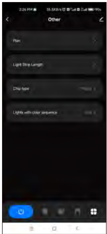
Other interface For the first time use, set LED strip length, chip type and color sequence.
